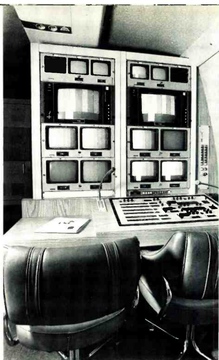
Production area of Channel One's Starshooter features an ISI 904 switcher and 3M digital matrix effects.
