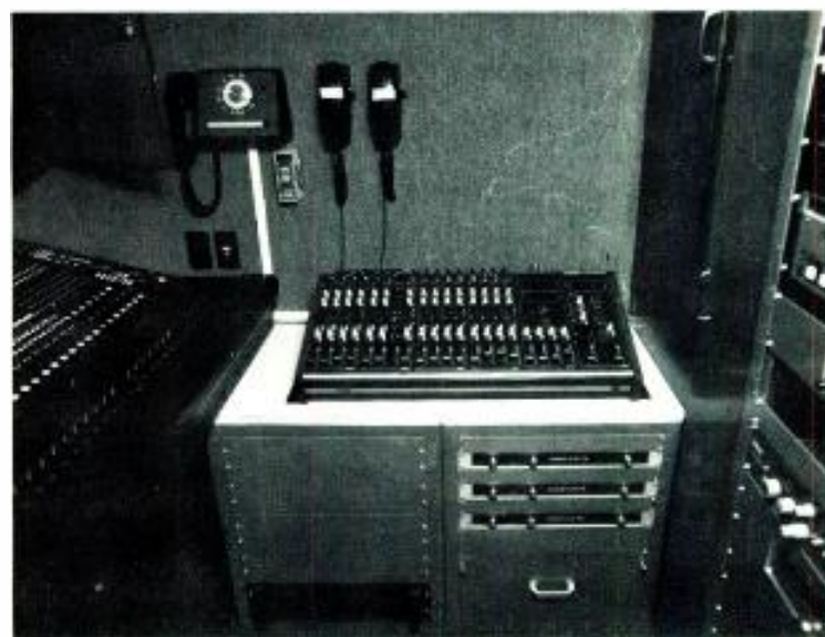
Quality Video's Tapco 16-input mixer, Crown amps, and Telex carts complete audio room in van.
